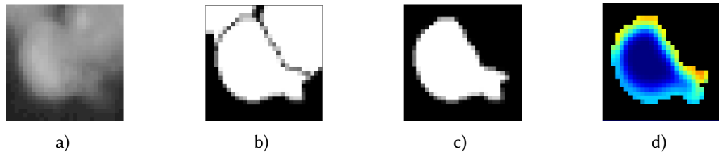
Figure 3.12: Weights for instances. For each box proposal, crops are resized to 28 \times 28 pixels. Crop from the input image (a), full-image segmentation mask (b), cell mask (c) and weight matrix (d).
