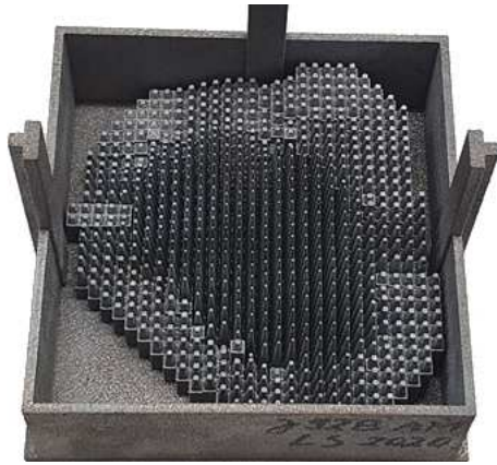
Figure 15. The aluminum 3D RM with a side wall and positioning bars. Figure taken from (Simeonov et al 2022) – Figure 5.
