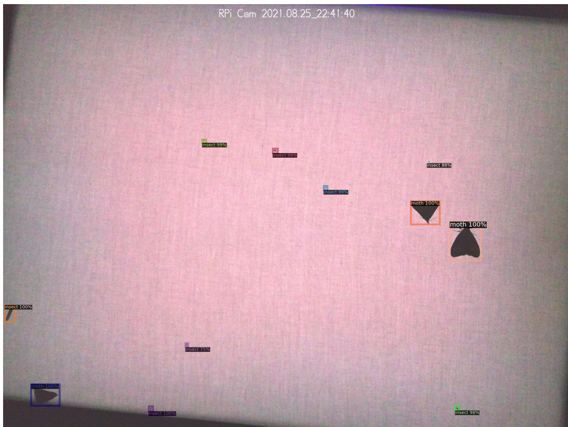
Fig. 3.12 Camera trap picture taken by AMT, with predicted bounding boxes around moths and insects.
