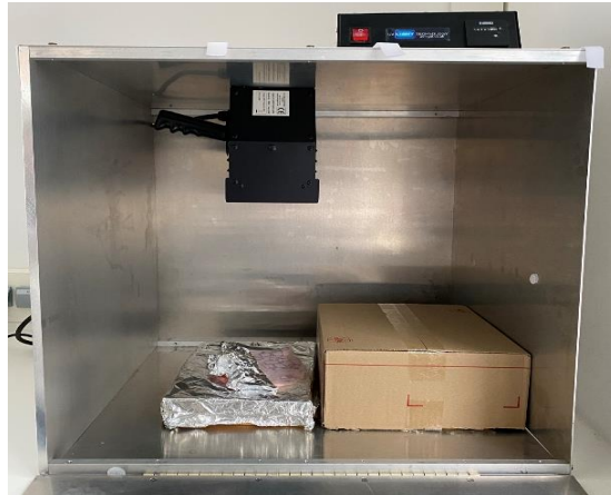
Figure 9: UV radiation source inside metallic box for exposure of the porcine skin
