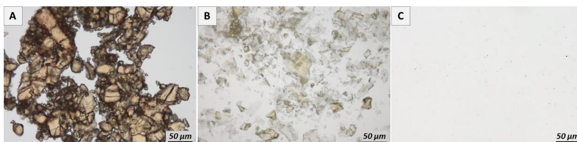
Figure 12: Microscopic images of BI-6C9 forming a lump in water (A), which was prevented by adding SDS solution (B) and transformed into a nanosuspension (C), each 400-fold magnification.
