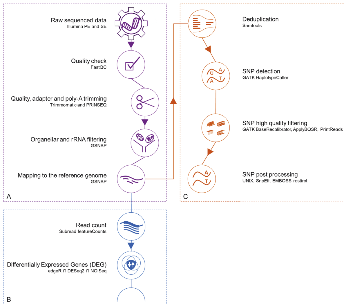
Figure 6: The RNA-seq pipeline design. The pipeline is structured in three functional units: A) RNA-seq pre-processing, includes sequence quality control, filtering and reference mapping, B) Gene expression calculation, normalization and DEG calling, and C) Variant detection/SNP calling.
