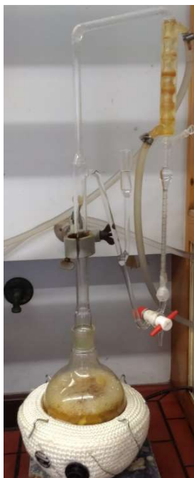
Figure 3-4 Extracting onion bulbs using a Clevenger apparatus.
