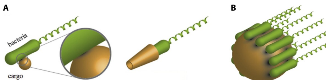
Figure 4 Attachment of single or multiple bacteria to synthetic cargo. Obtained and modified from Hosseinidoust, et al. (2016) 115 . Single-cell (A) and multi-cell (B) biohybrid systems with spherical or cone cargo.
