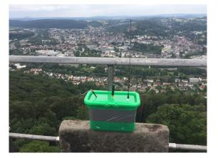
Figure 4.4: Waterproof static sensor box deployed.
