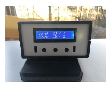
Figure 4.2: Base station for monitoring, relaying and processing.
