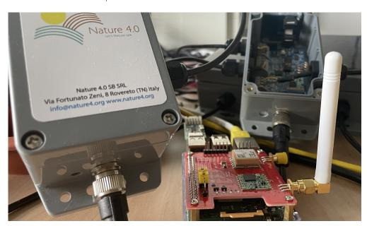
Figure 4.22: Original TreeTalker (left) and the ForestEdge hardware (right)
