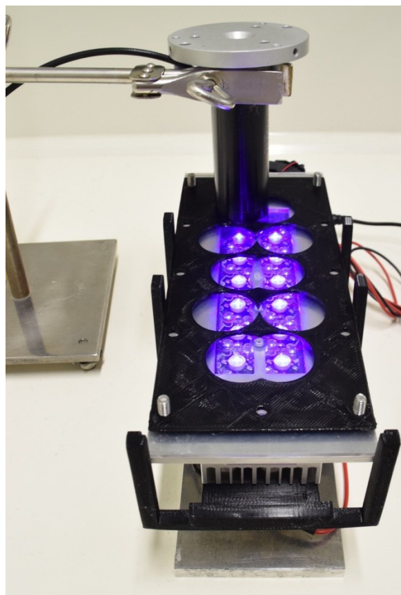
Figure 1.S16. Photograph of the final matching setup with the spectroradiometer fixed directly on the FEP foil and positioned by the 3D-printed scaffold.
