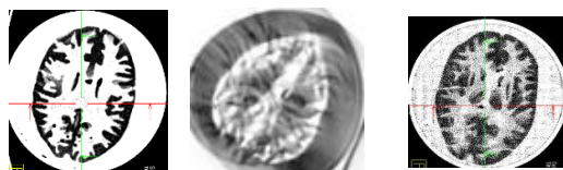
Figure 7.3: CT scan of a) stationary phantom, b) moving phantom, c) motion-corrected.
