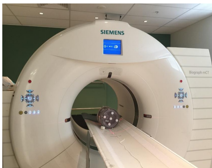
Figure 5.2: Hoffman brain phantom acquisition on Biograph mCT.
