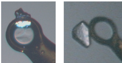
Fig. 1 Single crystals of heavy alkali metal triflates. Left: Colourless platelet of RbOTf and right: trapezoid-like crystal of CsOTf. Snaps recorded on an IPDS2T or IPDS2 diffractometer, respectively using X-AREA and applications therein.
